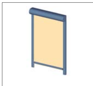
VB 106 - non-split fabric anti-glare blind, bar guided
