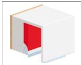
Insulation body with installation of Venetian blinds
