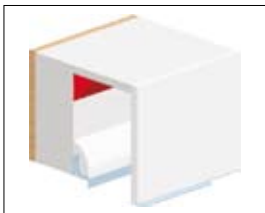
Insulation wedge with installation of roller shutters
